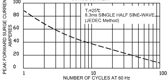
FIG.2 - MAXIMUM NON-REPETITIVE PEAK FORWARD SURGE CURRENT
